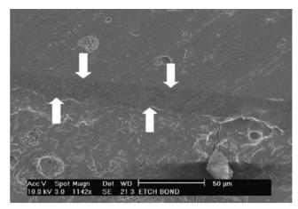
Fig 3. High resolution SEM of small tag of adhesive auto cure glass ionomer cement. Arrows show margins of resin bond between materials.
