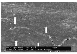
Fig 7. High resolution SEM showing interface of Riva LC RMGIC bond coated over auto cure glass ionomer cement prior to initial set and photo co-cured with composite resin. Arrows indicate interface of chemical RMGIC bond to GIC and composite resin.
