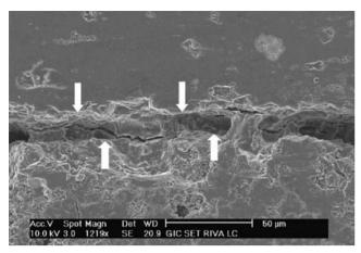
Fig 5. High resolution SEM showing interface of Riva LC RMGIC bond coated over set auto cure glass ionomer cement prior to applying and photo co-curing composite resin. Arrows show interface of RMGIC bond where the merged margins between GIC and composite resin suggest a chemical bond.
