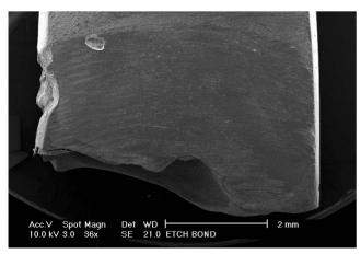
Fig 2. SEM of etched auto cure glass ionomer cement bonded to composite resin showing adhesive failure at interface.
